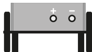
Figure 3 : Welding Cable Sockets
