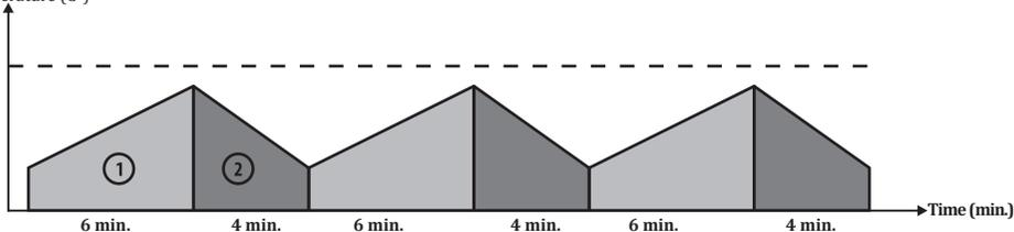
As defined in the standard EN 60974-1, the duty cycle rate includes a time period of 10 minutes. For example, if a machine specified as 250A at %60 is to be operated at 250A, the machine can weld / cut without interruption in the first 6 minutes of the 10 minutes period (zone 1). However, the following 4 minutes should be kept idle for the machine cool down (zone 2).
