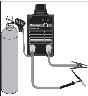
Figure 2 : TIG Welding Connections
